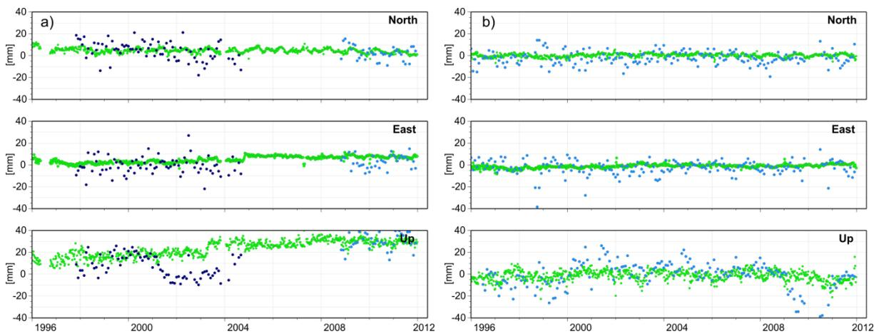
Fig. 8. Time series of  $N$ ,  $E$ ,  $U$  components of the GNSS station GRAS (green) and SLR stations 7835 (navy blue) and 7845 (blue) – on the left (a); time series of the WTZR (green) and SLR station 8834 (blue) – on the right (b)
