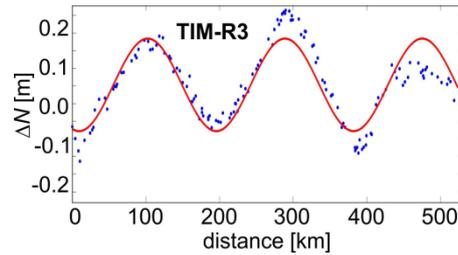
Fig. 1. Periodic pattern of the distribution of differences between the height anomalies from TIM-R3 and the corresponding ones from GPS/levelling at the control traverse
