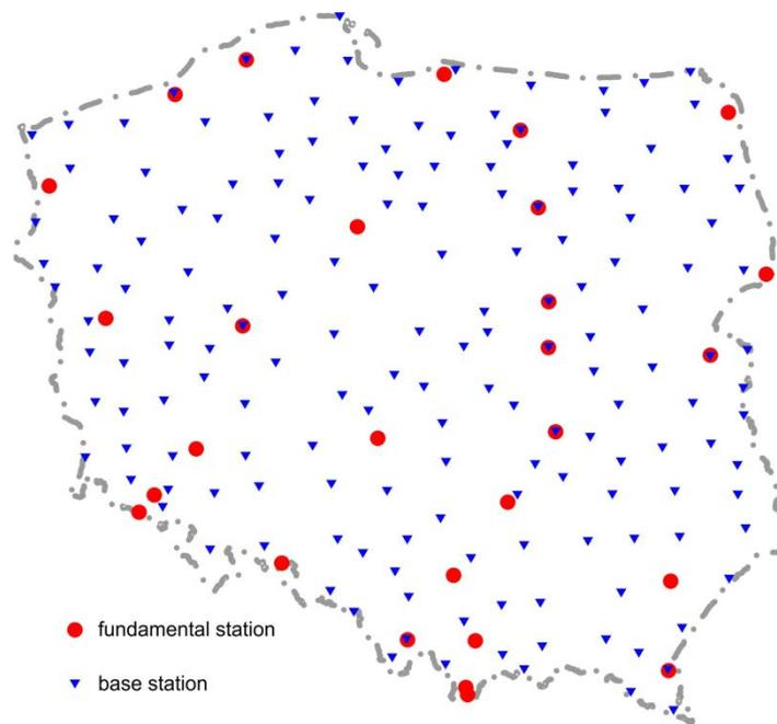
Fig. 18. Stations of new gravity control in Poland
