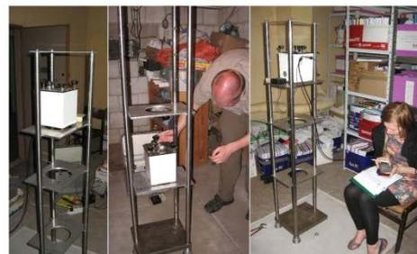
Fig. 20. The stand constructed by WUT (left) and IGiK (right) for vertical gravity gradient determination at field station and laboratory station, respectively
