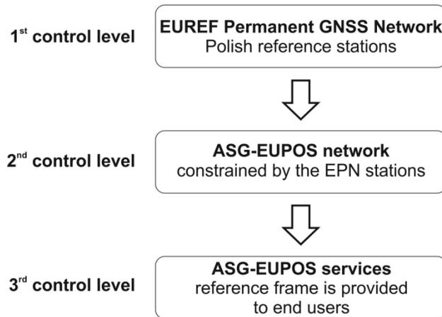
Fig. 13. ETRS89 realization and control via the ASG-EUPOS system
