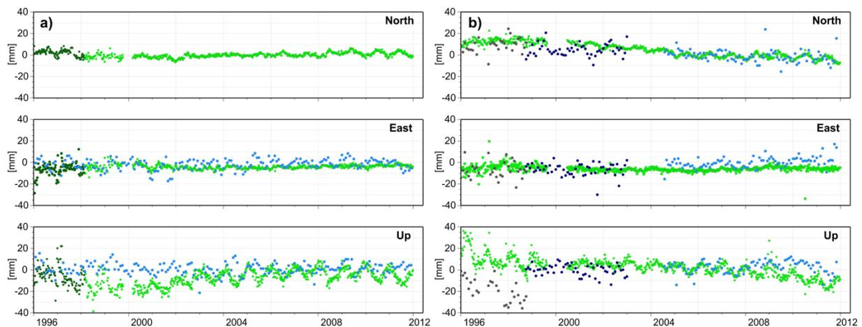
Fig. 9. Time series of  $N$ ,  $E$ ,  $U$  components of the GNSS stations YAR1 (grey) and YAR2 (green) and SLR station 7090 (blue) – on the left (a); time series of the GNSS station TIDB (green) and SLR stations 7843 (grey), 7849 (navy blue) and 7825 (blue) – on the right (b)
