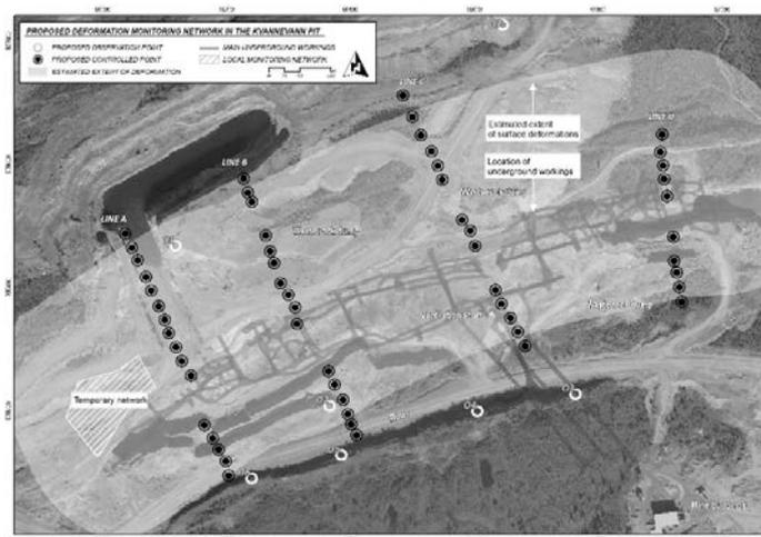
Fig. 18. Locations of controlled and observation points against the background of the production levels, estimated zone of deformation and surface features (Blachowski et al., 2011)
