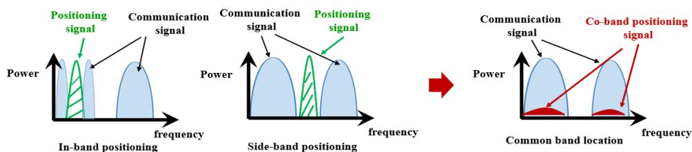
Figure 6. The principle of embedded signal-to-noise positioning
