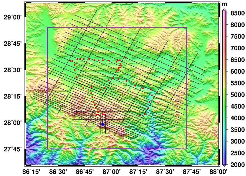
Figure 1. Airborne gravity survey lines and GNSS leveling points in the region of Mount Qomolangma (Blue triangle: Mount Qomolangma; Black Line: airborne gravity survey lines; Red point: GNSS leveling points; Purple rectangle: domain of quasigeoid model)
