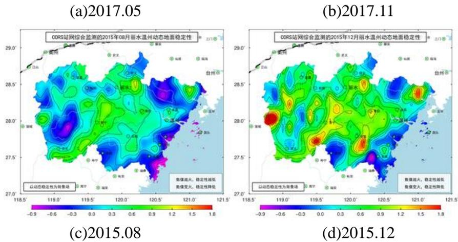
Figure 4. Comprehensive monitoring of dynamic ground stability in Lishui Wenzhou using CORS station network
