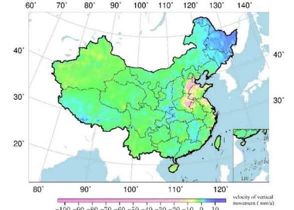
Figure 20. The vertical movement model of Chinese mainland by GNSS and Leveling data
