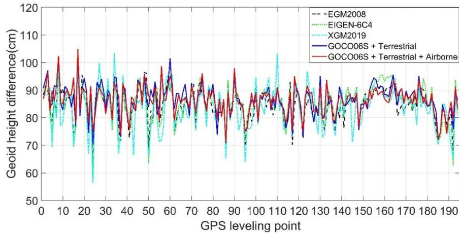
Figure 5. Differences between the gravimetric geoid models based on different data combination modes and the GPS leveling measured geoid heights. Results for EGM2008, EIGEN-6C4 and XGM2019 are included.
