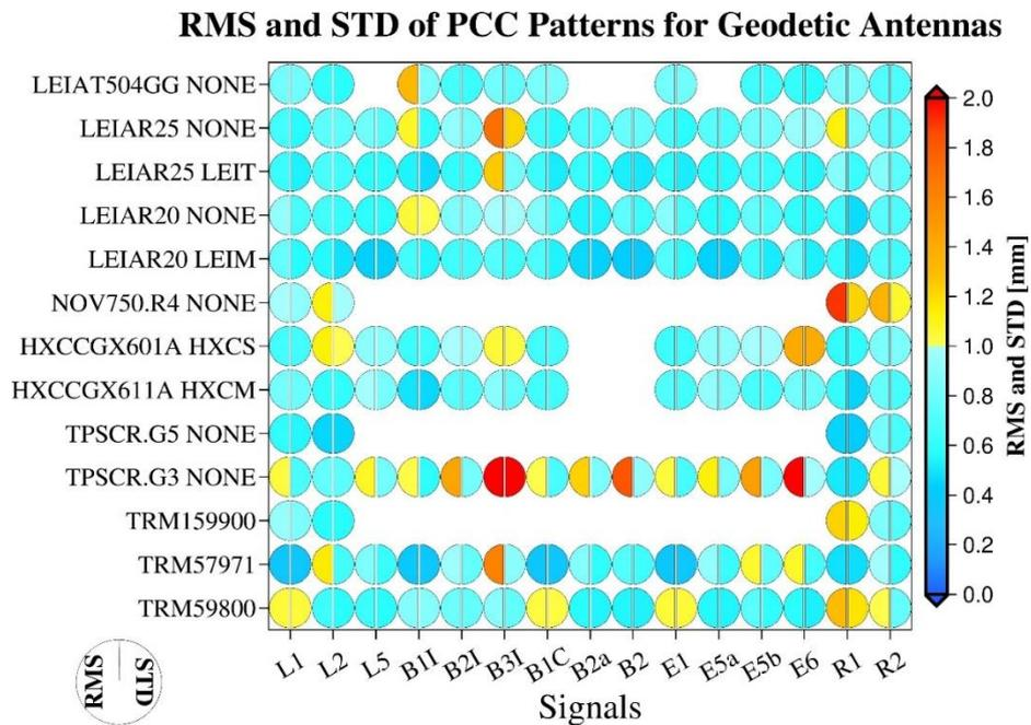
Figure 12. RMS Statistics of Antenna Phase Calibration for Different Antennas and Frequency Bands
