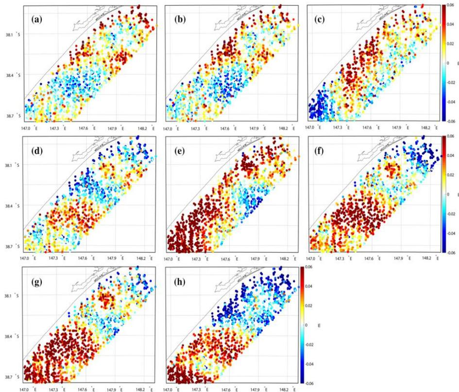
Figure 7. Evaluations of different gravimetric quasi-geoid models with the altimeter-derived quasi-geoid heights only located within the boundary of airborne survey. a QGland\_TSA, b QGland\_TS, c AGQG2017, d EGM2008, e EIGEN-6C4, f GECO, g SGG-UGM-1 and h GOCO05c. Note that the mean values of the misfit between gravimetric quasi-geoid models and altimeter-derived data are removed.
