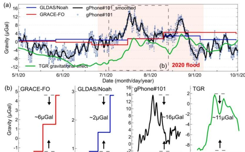
Figure3. The different gravity sensors and model, at gPhone#101 location, response to TWS changes in TGR during 2020 flood season (Wang et al., 2021).
