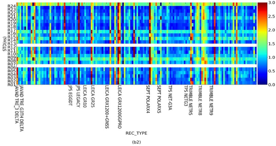
Figure 6. The mean value (a) and the STD (b) for GLONASS IFB (1:  $IFB_1$ ; 2:  $IFB_2$ ) of each receiver-satellite pair for IGS stations in March 2017 based on the undifferenced and uncombined PPP solution. The X-axis is grouped according to the receiver type. The color bar represents the STD value in ns, and the averaged STD is about 1.107 ns
