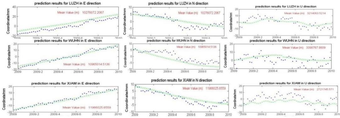
Figure 10. Prediction results for station nonlinear movements in the N, E, and U directions in the South China subplate.
