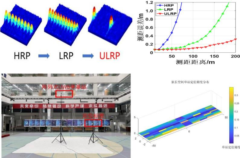
Figure 4. The proposed novel UWB signal system suitable for underground space and experimental results
