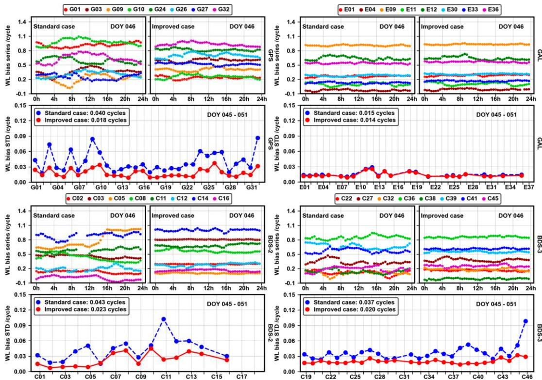
Figure 3. WL phase bias series on DOY 46, 2021 and the corresponding STDs across 7 days for GPS, Galileo, BDS-2, and BDS-3 before and after the calibration of signal distortion biases
