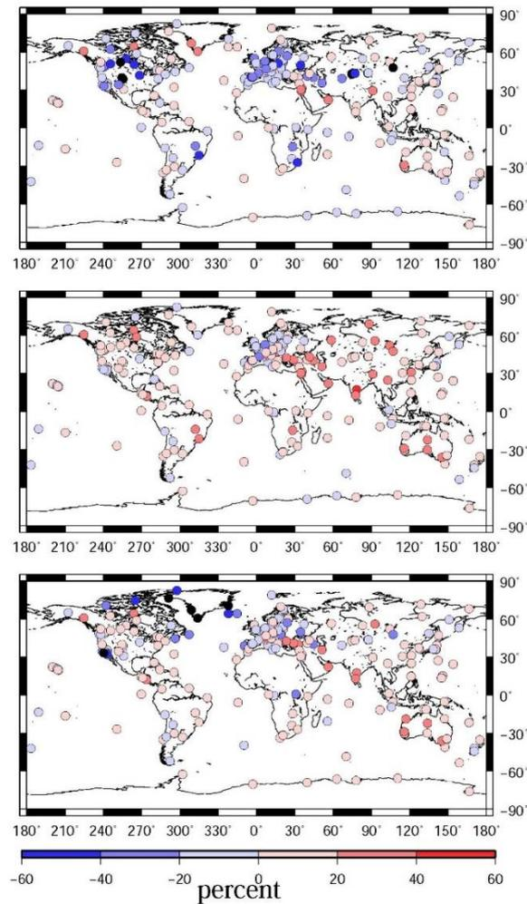
Figure 13. Spatial distribution of WRMS differences in percentage using the three loading corrections. Black circles indicate that a station's WRMS change exceeded the limits of the scale range. Unit of WRMS difference is %. Top panel shows the QLM model; the middle panel shows the OMD model; the bottom panel shows the GGFC model.
