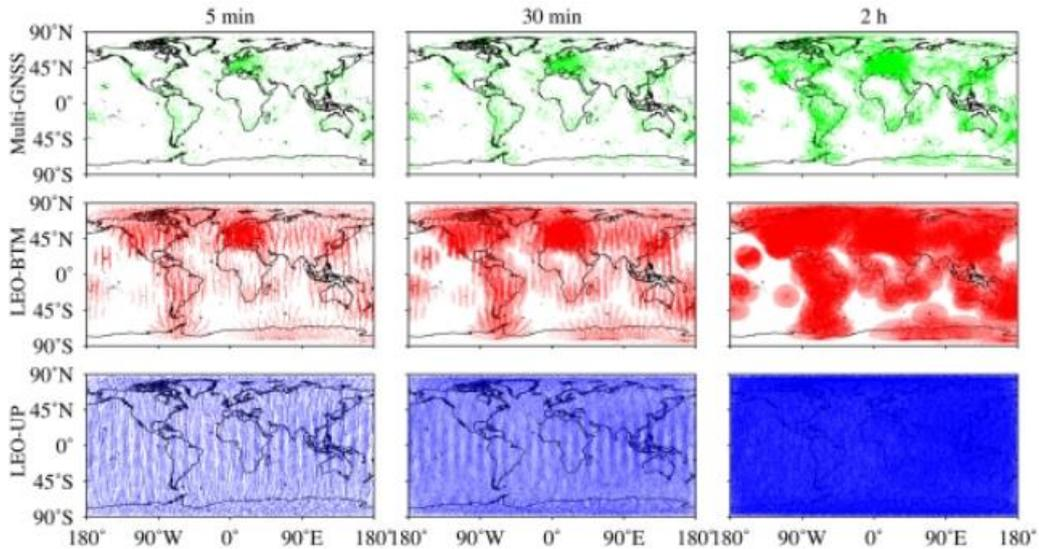
Figure 3. Distribution of ionospheric pierce points derived from Low-Earth-Orbiting (LEO) constellation with 192 satellites within different time spans, that is, 5 min, 30 min, and 2 hours, respectively.
