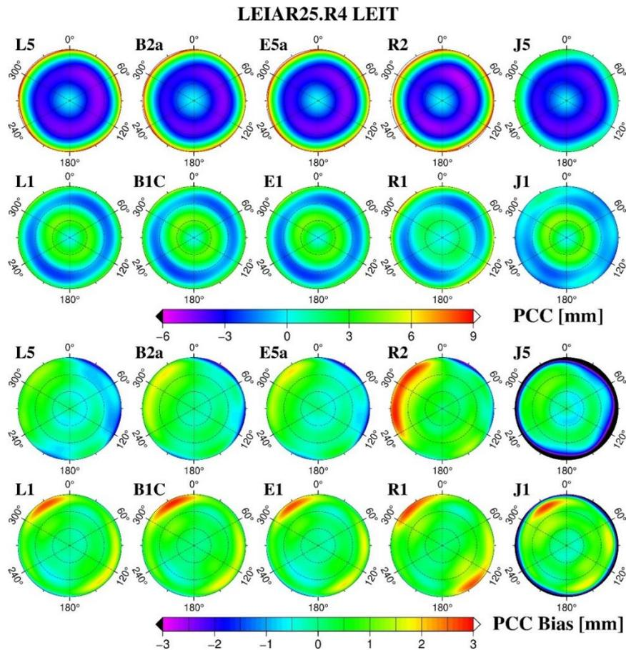
Figure 11. Calibration accuracy for different signals of LEIAR25.R4 LEIT, compared with igs14.atx. The differences are calculated in a grid format.
