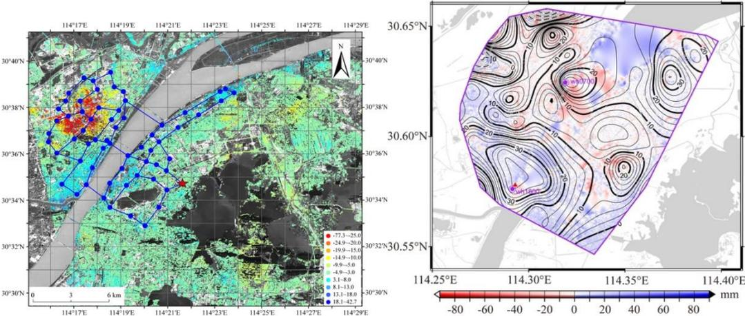
Figure 4. Left: Surface subsidence observed by InSAR and the mobile gravity observing network, Blue dots are gravity points. Red ★ point is the absolute gravity control point. Right: Comparison of the gravity change from the 1st campaign to the 7th covered on the vertical displacement observed by D-InSAR (Chen et al., 2020)
