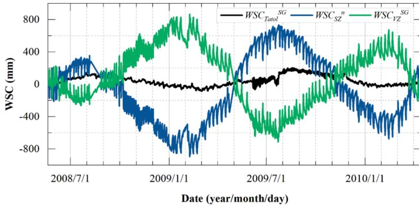
Figure2. Water storage changes at Wuhan SG Station quantitatively separated using the superconducting gravity technique. (He et al., 2022)
