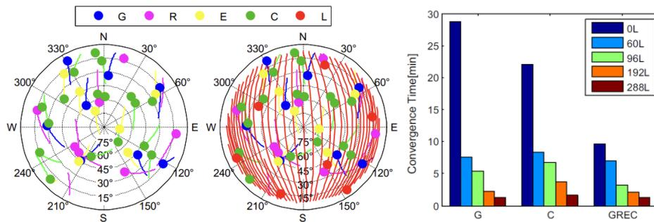
Figure 7. Sky plots of the multi-GNSS satellites without or with the augmentation of 192 LEO satellites (left panel); Average convergence time of LEO augmented PPP solutions(right panel)
