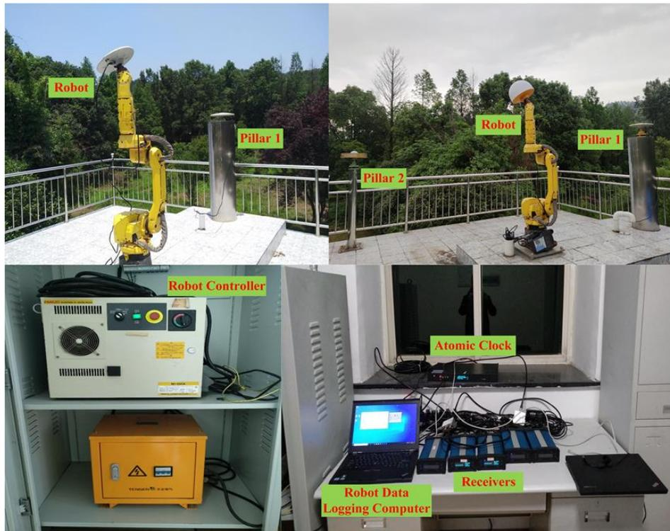
Figure 10. Field antenna calibration system at Wuhan University. The system is built on a rooftop and includes a six-axis robot, a controller, an atomic clock, receivers and other auxiliary equipment.
