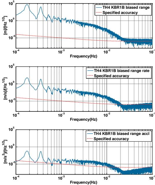
Figure 12. The spectrum of KBR biased range, range rate and range acceleration in the dual-one way ranging
