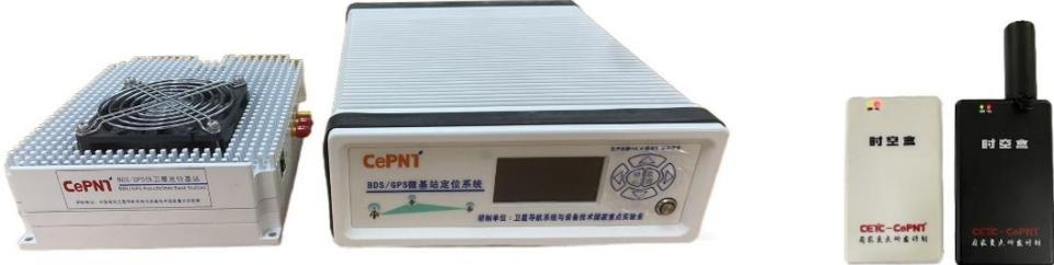
Figure 1. Beidou pseudosatellite indoor positioning micro base station and positioning terminal "spatiotemporal box"
