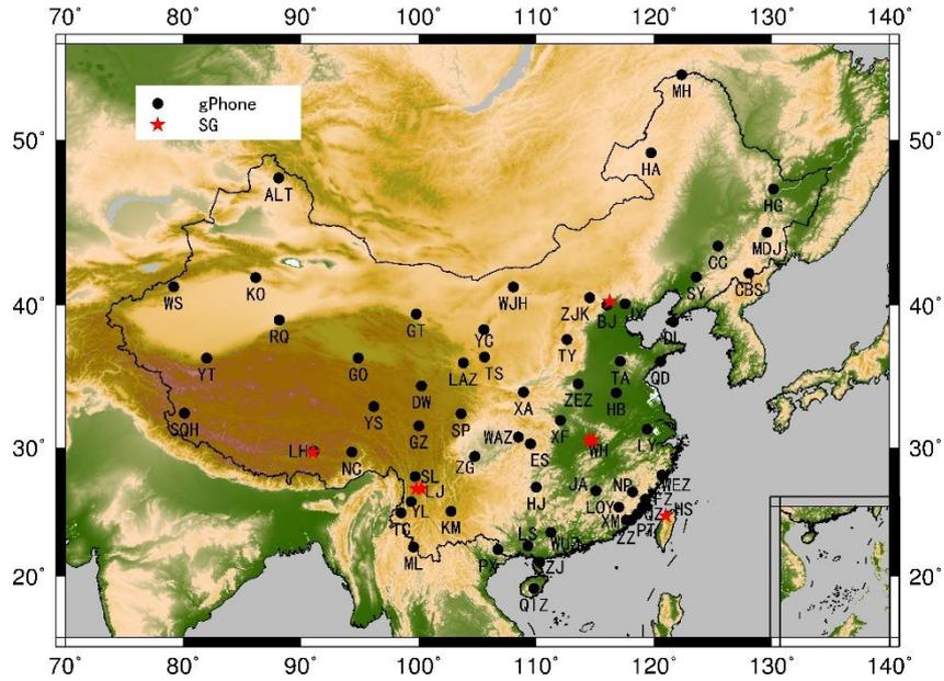
Figure 1. The distribution of 60 gPhone gravimeters and 7 Superconducting gravimeters (SGs: Wuhan (2), Lijiang (2), Lhasa (1), Beijing (1) and Hsinchu (1)) over China's mainland. gPhone stations are represented by the black solid circles while SG stations are represented by the red solid stars (Sun et al., 2022).
