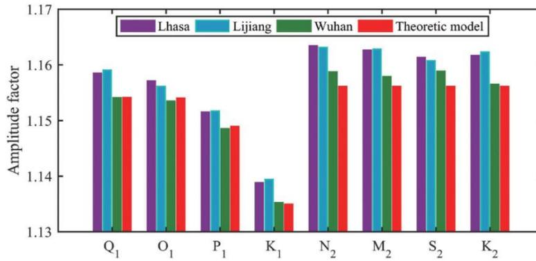
Figure 3. Comparison of the amplitude factors of diurnal and semidiurnal tidal waves observed in Lhasa, Lijiang, and Wuhan SG stations and the theoretical values from Mathews's (2001) model (Sun et al., 2019b).
