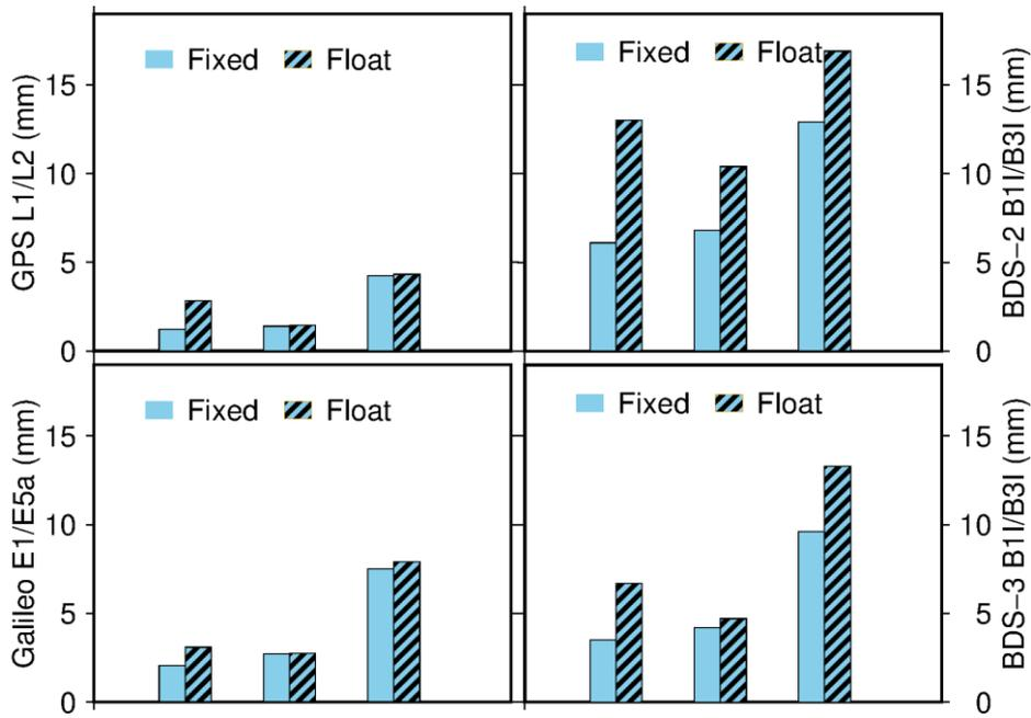
Figure 8. RMSE at E, N, and U directions of float and fixed solutions for single-system dual-frequency PPP-AR using WUM rapid phase bias products
