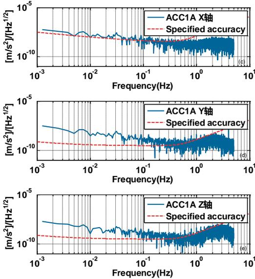
Figure 13. The accelerometer high-sensitive axis noise level being  $3 \times 10^{-10} \text{m/s}^2/\sqrt{\text{Hz}}$  near the frequency 0.1Hz, and being  $1 \times 10^{-9} \text{m/s}^2/\sqrt{\text{Hz}}$  for the less-sensitive axis
