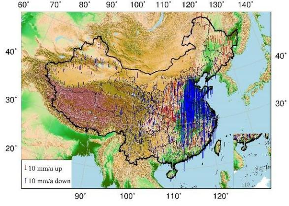
Figure 19. Vertical Velocity of GNSS Points
