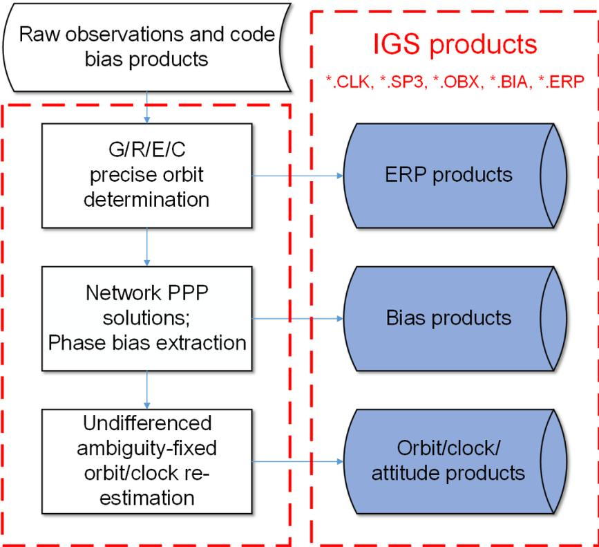
Figure 7. Flowchart of WUM rapid phase clock/bias and orbit products generation procedure. Blue boxes depict the estimated products. G, R, E, C represent GPS, GLONASS, Galileo, BDS respectively
