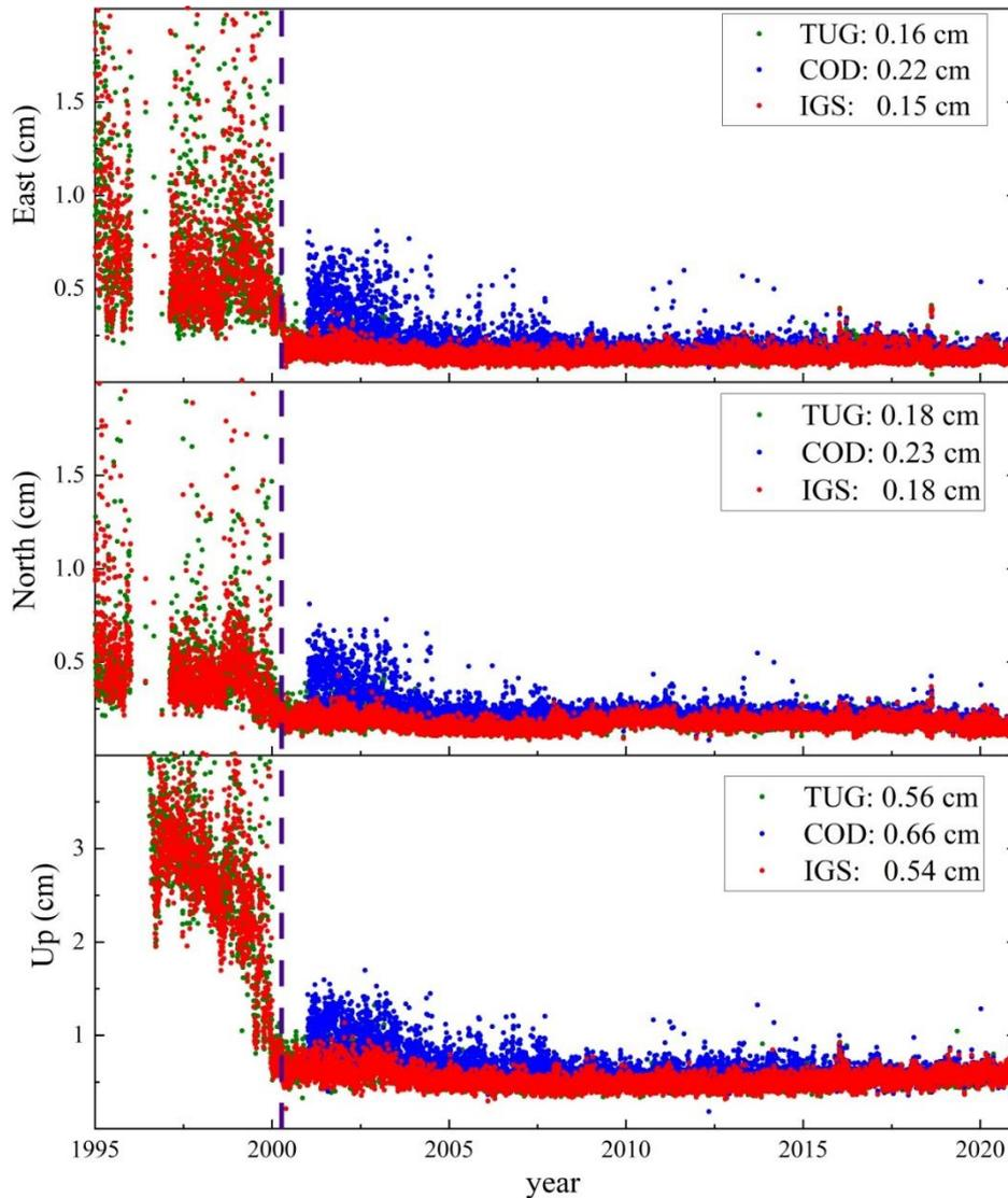
Figure 9. Positioning accuracy comparison between combined phase clock/bias products and individual AC products. The vertical dashed line in each subfigure denotes the date that GPS abandoned the “Selective Availability” policy.
