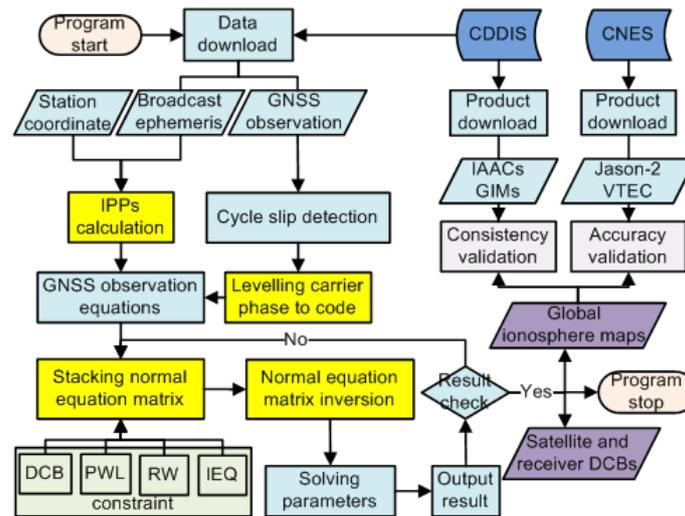
Figure 3. The GIMAS software flowchart.
