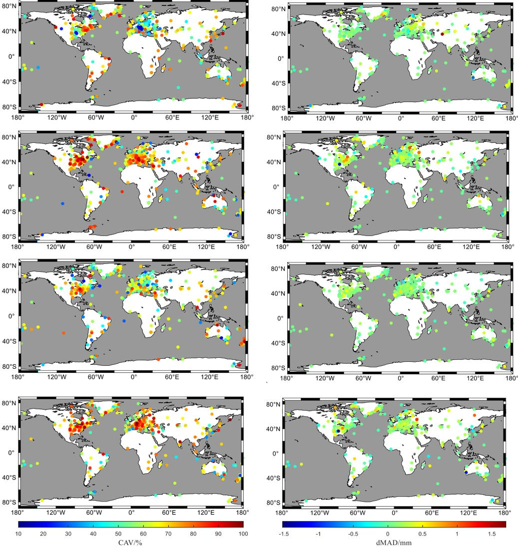
Figure 2. Spatial distribution of CAV (consistency of amplitude variation) of the annual signals between the environmental loading and coordinate time series (left) and the change of MAD (mean absolute deviation) (right). From top to bottom are ATML, CWSL, NTOL and total environmental loading
