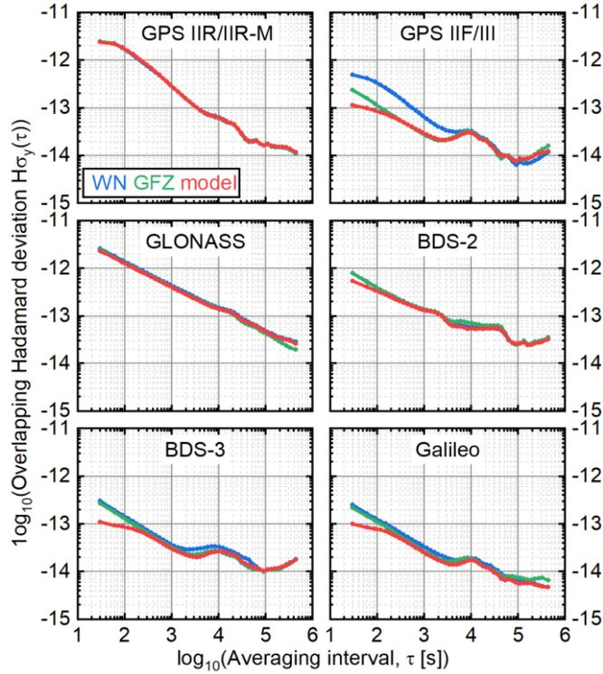
Figure 5. Overlapping HDEV of the estimated clock products with the WN (white noise) and model (clock model). Average values for different sets of clocks were calculated based on products from GPS week 2177–2183. Also, the results of GFZ final multi-GNSS products (green) for the same period were shown as references
