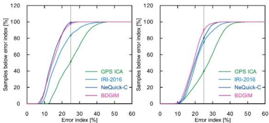
Figure 1. Cumulative distribution of different correction model errors compared to IGS-GIM (left) and Jason VTECs (right) covering solar maximum and minimum conditions. The vertical line denotes the targeted 25% error index (adapted from Wang et al. 2020).
