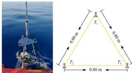
Figure.1 Schematic diggram of seafloor control point and beacon placement position on the station
