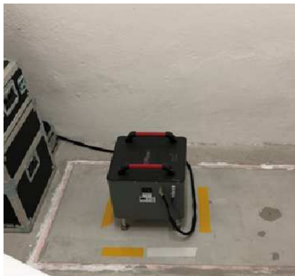
Fig. 2: Relative metal spring gravimeter gPhoneX #108 in Hurbanovo station.
