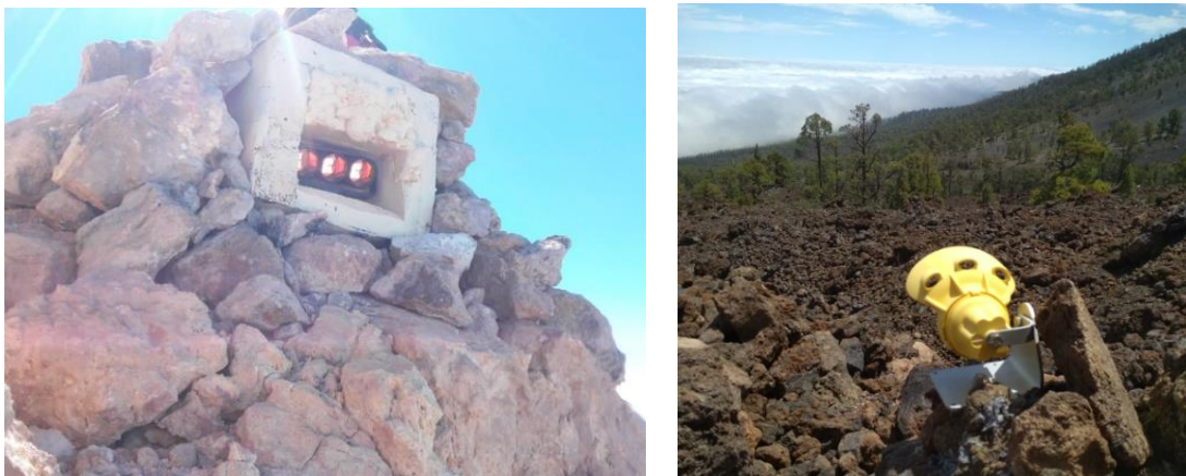
Multiparametric station (up) and prisms (down)
