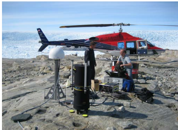
Absolute gravity measurement at GNET site in East Greenland
