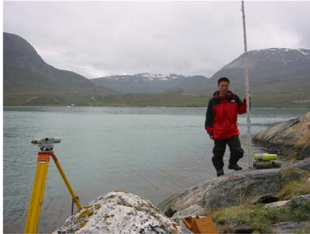
Fjord height and tide measurement in Greenland to support geoid determination
