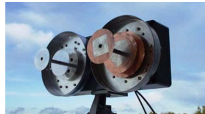
The field-of-view at the observation site and the L1 and L2 receiving antenna array.
