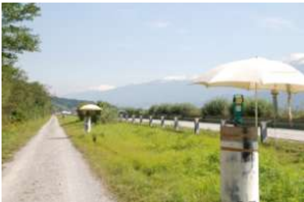
Figure V-3. The geodetic baseline of the BEV in Innsbruck, Austria. (Photo: Jorma Jokela)
