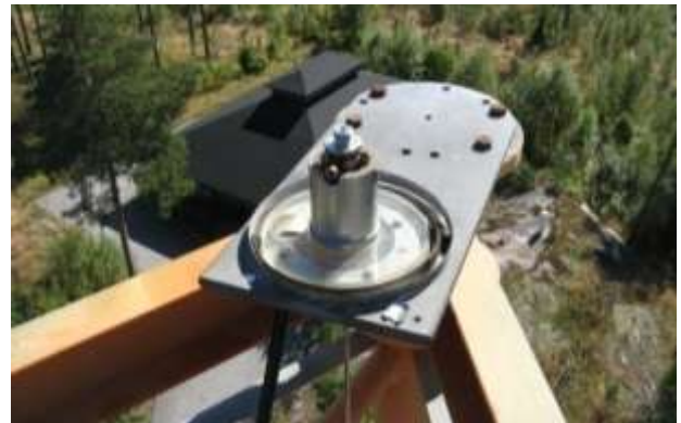
Figure I-6. The antenna on top of the 20 m high steel grid mast is stabilized with a special invar wire construction which eliminates the thermal expansion of the mast. (Photo: Hannu Koivula)
