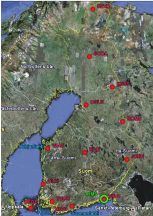
Figure IV-3. The FinnRef ® network of permanent GPS stations (red circles) and the EGNOS RIMS station (green open circle) in GoogleEarth ™ .
