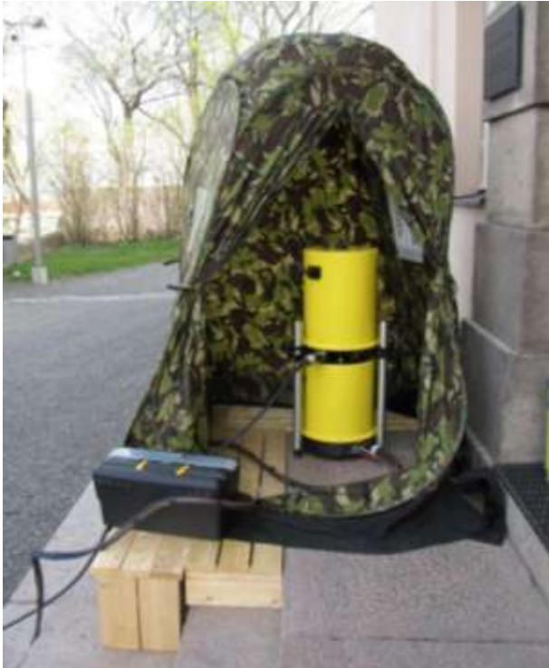
Figure II-9. The A10-020 at the station Turku Vartiouuri. Note the transportable benches and weights to mount the tent on stairs. (Photo: Jaakko Mäkinen)
