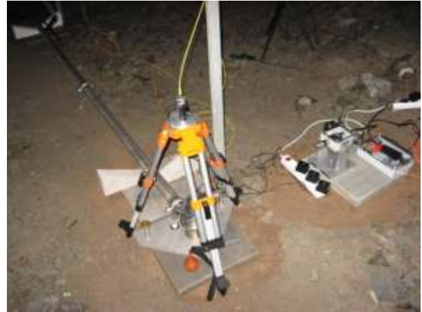
Figure III-5. The Fizeau-Kukkamäki liquid level interferometer in the north end of the NSWT. (Photo: Hannu Ruotsalainen)
