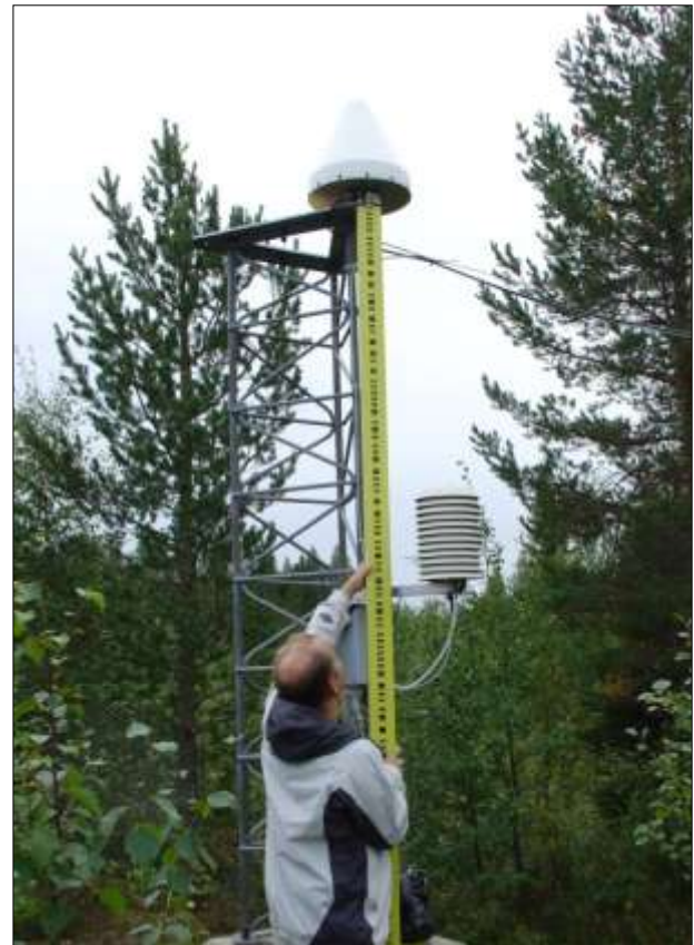
Figure I-5. Control measurement of the mast of the permanent GPS station. The stations are monitored independently from GNSS with precision tacheometry and precise levelling. (Photo: Olli Wilkman)
