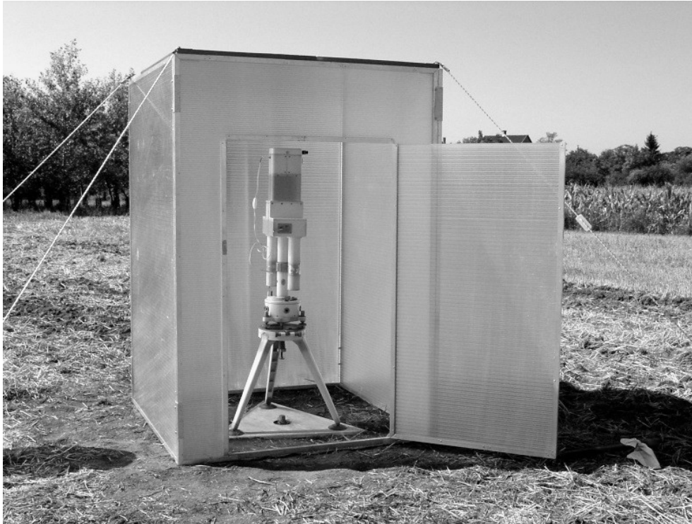
Fig. 3. Torsion balance measurement by E54 instrument on the Csepel Island.
