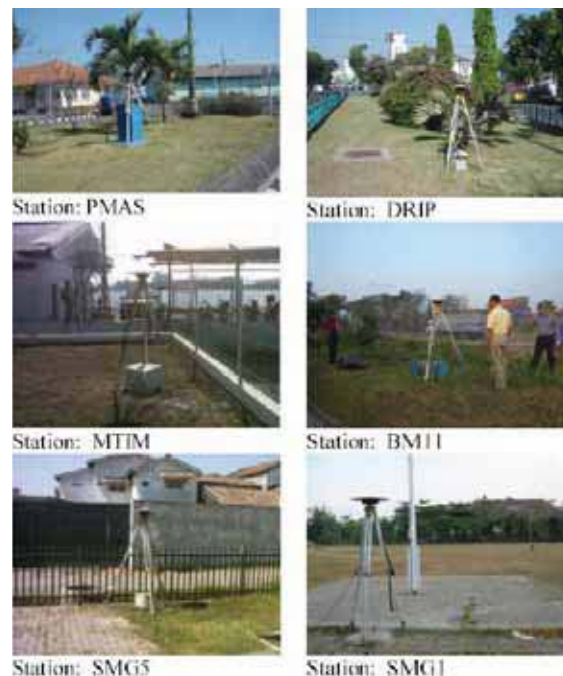
Figure 9. Example of GPS stations for monitoring land subsidence in
