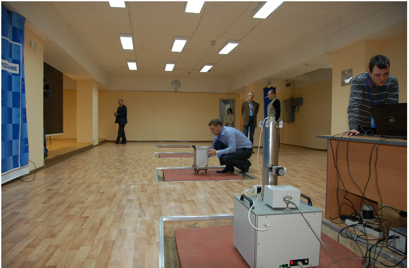
Fig. 5 Comparison of absolute gravity meters at the site of East Siberian Division of the Federal Service of Registration, Cadastre and Cartography
