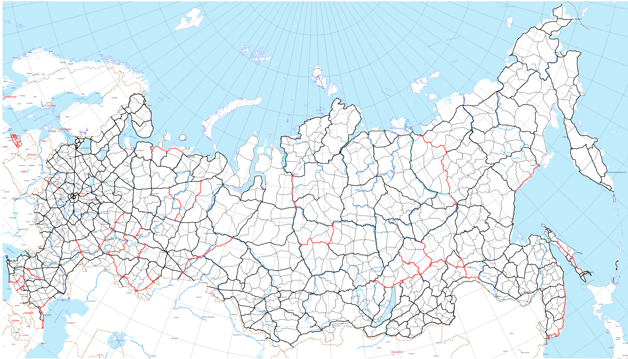
Fig.2. Main Russian Vertical Reference Frame (first order leveling – solid, second order leveling – thin, planned - red)
