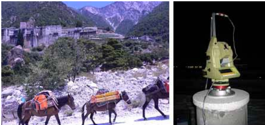
Figure 4.74: Transport of the material to Holy Mount Athos (left). The buildings in the background belong to the Monastery Agios Pavlos (Saint Paul). TCA1800 Total station with DAEDALUS system mounted (right).
