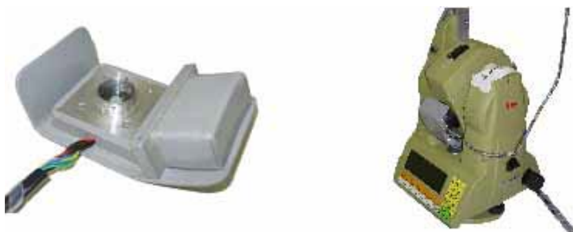
Figure 4.80: Transformed CCD camera and the mechanical Leica interface (aluminum plate, left picture). The right picture shows the camera mounted on a TCA 1800. This flat layout allows to measure in zenith direction.
