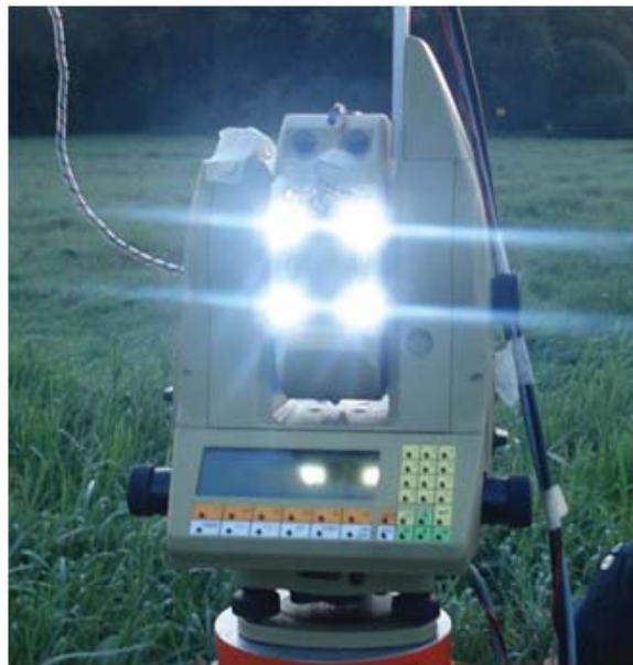
Figure 4.84: Leica TCA 1800 Total Station equipped with DAEDALUS and additional four power diodes symmetrically arranged around the telescope. Two total stations equipped this way enable centered reciprocal vertical angle measurements.
