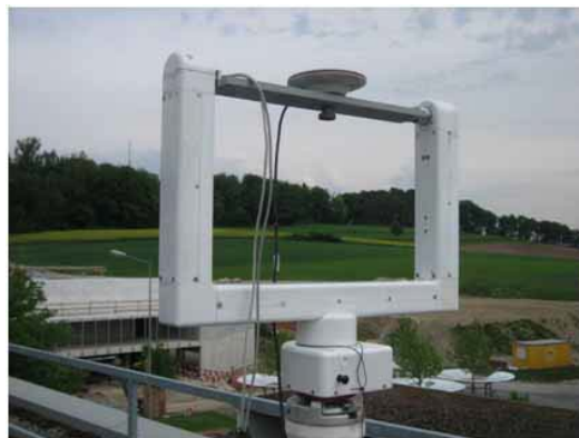
Figure 4.69: Measurement setup with the rotation simulator and the mounted GPS antenna.
