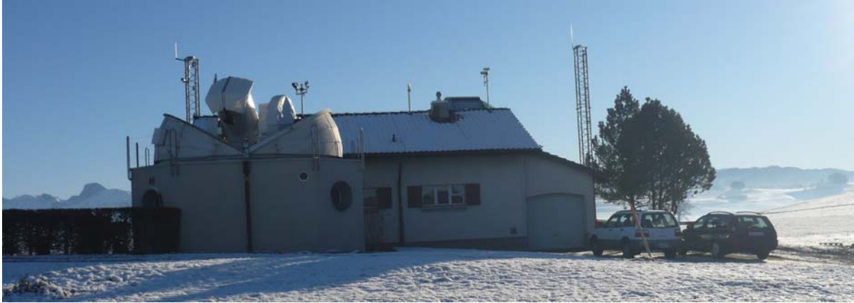
Figure 1.15: The Zimmerwald Observatory with the monostatic 1-m laser and astrometric Telescope ZIMLAT (foreground), the 9-meter masts of the GPS-only station ZIMM (left) and the GPS/GLONASS station ZIM2 (right).
