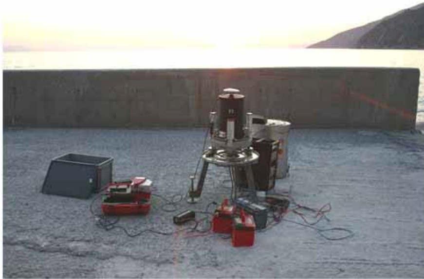
Figure 4.73: The zenith camera system DIADEM near the Monastery Agios Pavlos (Athos). Prior to the observations to the stars, the geodetic coordinates are determined with a GNSS receiver (visible on top of the camera).
