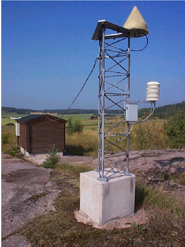
Fig. 2. The permanent GPS station of Virolahti. (Photo: Ruizhi Chen)
