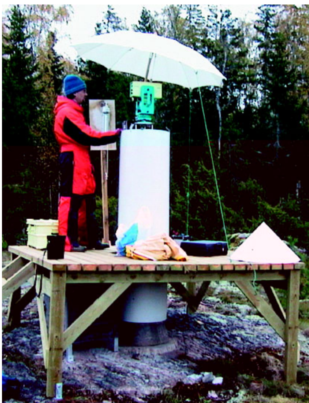
Fig. 2. Controlling the scale of a local GPS network for deformation studies with high precision EDM. (Photo S. Ahola)
