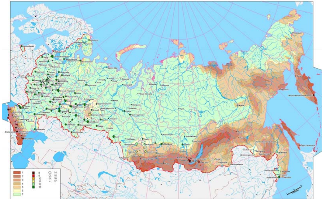
Fig. 6.1. Zonation of the Russian Federation territory according to the level of seismic risk R_e , 10^{-5} 1/year categories: 1- extremely high; 2 – rather high; 3 - high; 4 – average; 5 - moderate; 6- insignificant; 7 - low. Values of risk for the cities with population more than 50 000 people, R_e , 10^{-5} 1/year: 8 – 20 up to 50; 9 – 10 up to 20; 10 – 5 up to 10; 11 – 1 up to 5; 12 – 0.5 up to 1; 13 - less than 0.5. Number of inhabitants: 14 –1 000 000 and more; 15 - 500 00 up to 1000 000; 16 – 200 000 up to 500 000; 17 – less than 200 000
