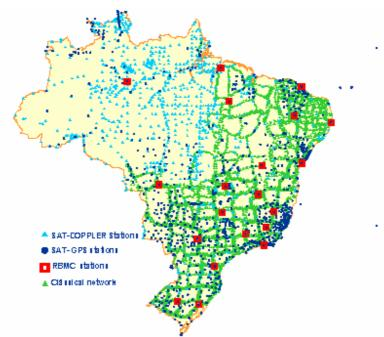
Figure 7 - Geodetic Network adjusted in 2006
