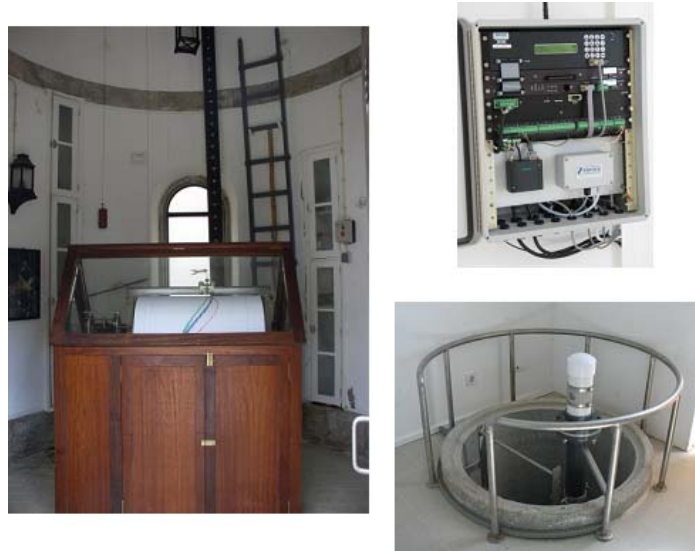
Figure 2.5 – Cascais Tide Gauges. Left: Borel Floating System. Right: Acoustic.
