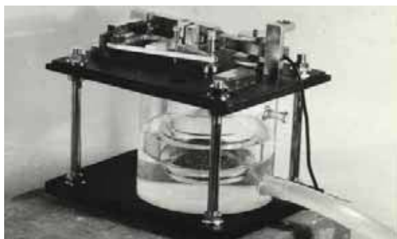
Figure 2. Water-tube tiltmeter (single terminal)
