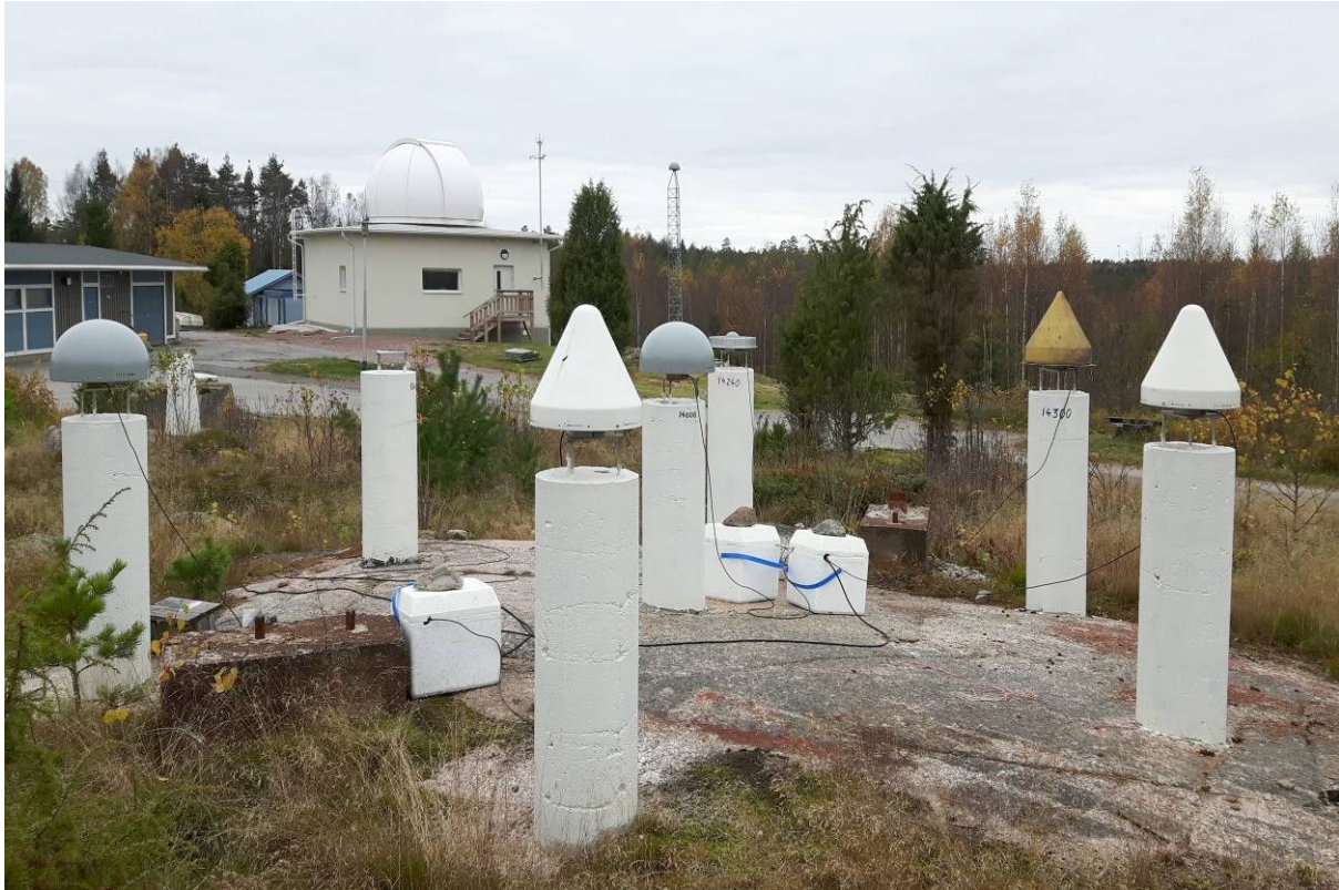
A GNSS antenna test field in Metsähovi. The dome of the new SLR telescope is at background. (Photo: M. Poutanen / FGI)
