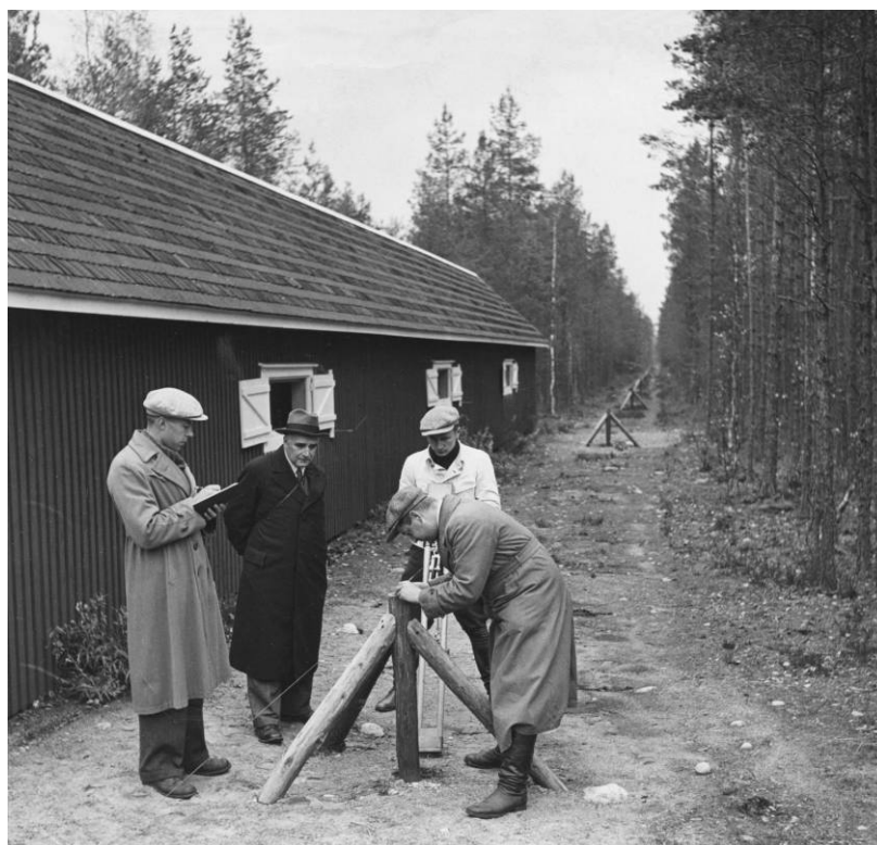
Calibration of invar wires at the Nummela Standard Baseline in 1939. (Photo: FGI archives)
