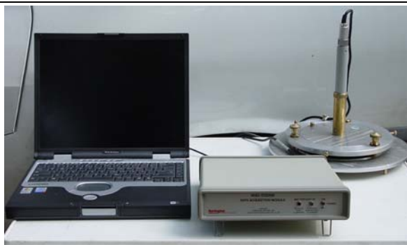
Fig. 8. MAG-03DAM acquisition module with 6 channel, 24 bit resolution, sampling rate programmable, internal and external battery of 12 V
