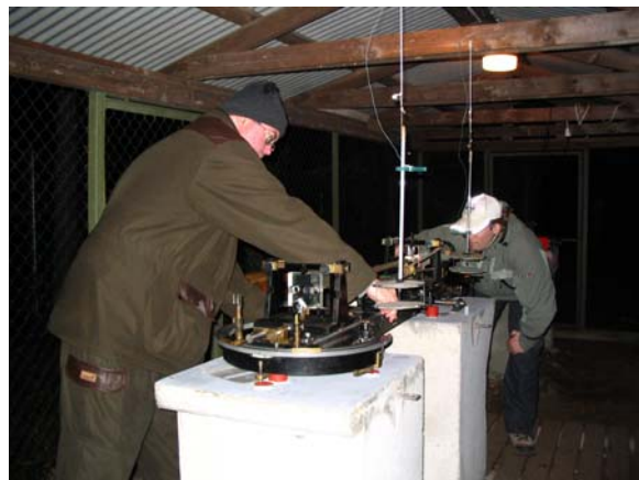
Fig. 33. Väisälä interference measurements at the Nummela Standard baseline. Photo Pasi Häkli.
