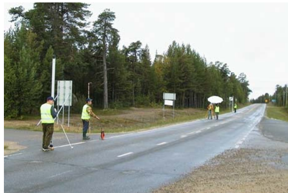
Fig 5. Field work of the Third precise levelling of Finland. Photo Markku Poutanen.
