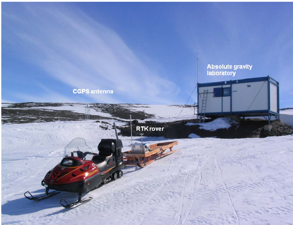
Fig. 25. Absolute gravity laboratory and permanent GPS station at the Finnish Antarctic base Aboa. Photo Joel Ahola.
